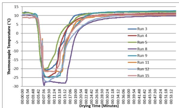
Plot of product temperature for a group of DoE experiments over the primary drying cycle.
