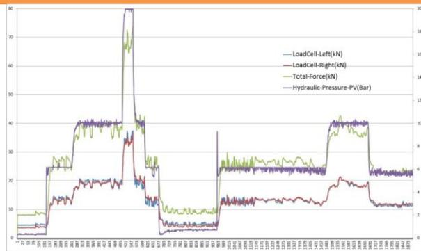
When studying the roller compaction of a powder mixture, the process parameters are available on screen and can be investigated in more detail subsequently. In the two images below, the roll gap and load cell forces are shown for an experimental run
