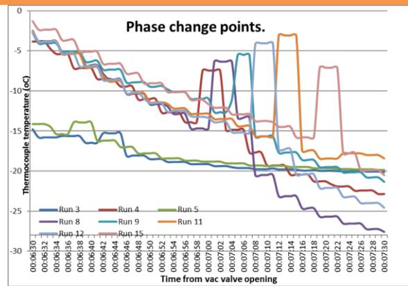
Fine filament thermocouples allows observation of the increase in temperature on product freezing
