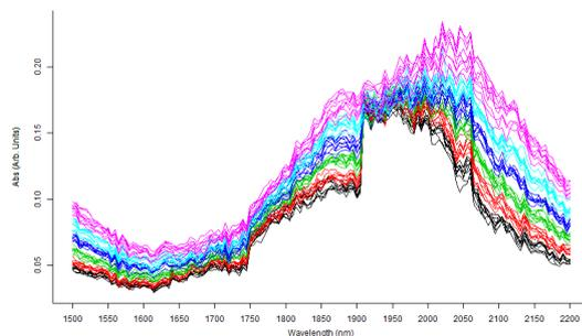
Training spectra from four probes in reflection mode when compaction pressure is increased from 5 to 30 Bar in 5 Bar steps. Baseline shifts upwards with increasing pressure.
