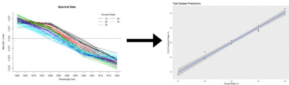
Measurement of each vial of powder takes less than one second, applying some advanced data analysis allows water content to be predicted. The graph on the right shows the predicted vs the measured (by reference method) values. The Error is within 5 %
