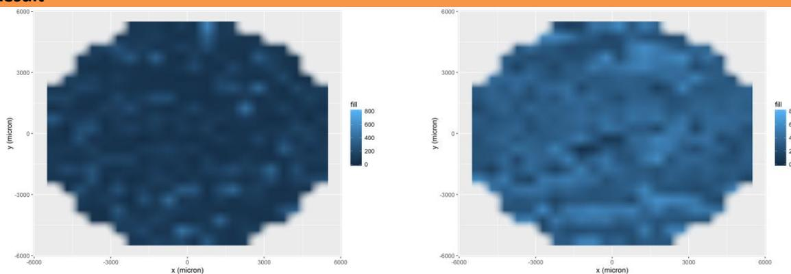
The images show tablets with 20 (left) and 70 (right) % by weight of API, the lighter blue indicates a higher concentration of API. Domains of higher API concentration can be observed in the right hand image, suggesting that the API may stick together when flowing into the tableting machine.
