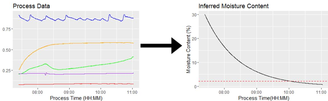
The image on the left is typical of what is produced during manufacturing processes, the information is hard to decipher. Analysing the signals using mathematical and statistical methodologies allows the image on the right to be produced. This shows much more relevant information from a process standpoint (*i.e.* the correct moisture content was reached at 10:00). The algorithms used are often lightweight enough to be implemented in real time.
